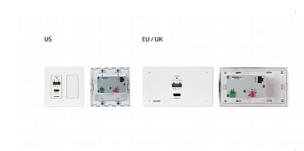
WP-789R is a high-performance, long-reach HDBaseT wall-plate receiver for 4K@60Hz (4:2:0) HDMI and HDCP 2.2 signals over twisted pair. It converts the transmitted HDBaseT signal into an HDMI signal. It extends video signals up to 40m (130ft) over Kramer copper cables at 4K@60Hz (4:2:0) 24bpp video resolution and provides even further reach for lower HD video resolutions. This wall-plate is powered through PoE (Power over Ethernet) over the twisted pair cable
