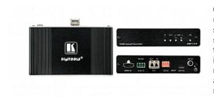
676T is a high-performance HDMI fiber transmitter for ultra-reach extension of 4K@60Hz (4:4:4) HDMI signals. 676T converts the HDMI and RS-232 input signal to an optical signal that is transmitted over a fiber optic cable to a compatible receiver that converts it back to HDMI and RS-232 signals. 676T includes a multi-mode SFP+ transceiver, but can be used with any Kramer certified SFP+ transceiver, such as a single-mode SFP+ transceiver
