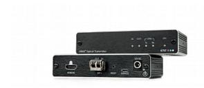
675R/T is a high-performance HDMI fiber extender kit for ultra-reach extension of 4K@60Hz (4:4:4) HDMI signals. 675T converts the HDMI input signal to an optical signal that is transmitted over a fiber optic cable to 675R, which converts it back to an HDMI signal. 675R/T includes 2 multi-mode SFP+ transceivers, but can be used with any Kramer certified SFP+ transceiver, such as a single-mode SFP+ transceiver
