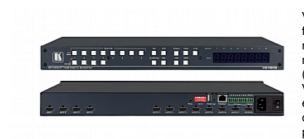
VS-48H2 is a high-performance 4x8 matrix switcher for 4K@60Hz (4:4:4) HDR signals and digital audio routing. It reclocks and equalizes the signals and can route any one of 4 HDMI, HDCP-compliant sources (selectable) to any or all outputs simultaneously. VS-48H2 offers unmatched audio flexibility where any embedded digital audio input can be routed to any digital output in addition to eight ARC sources to produce an equivalent 12x12 audio matrix
