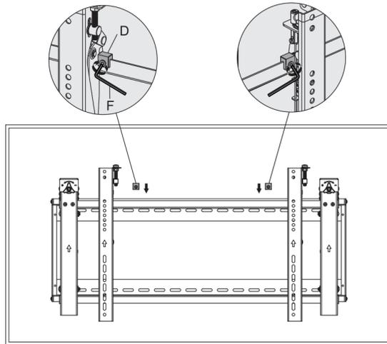
Install the both antiskid blocks as close to the adapter brackets as possible. Tighten screws on the antiskid blocks using an Allen key to prevent display from moving.
