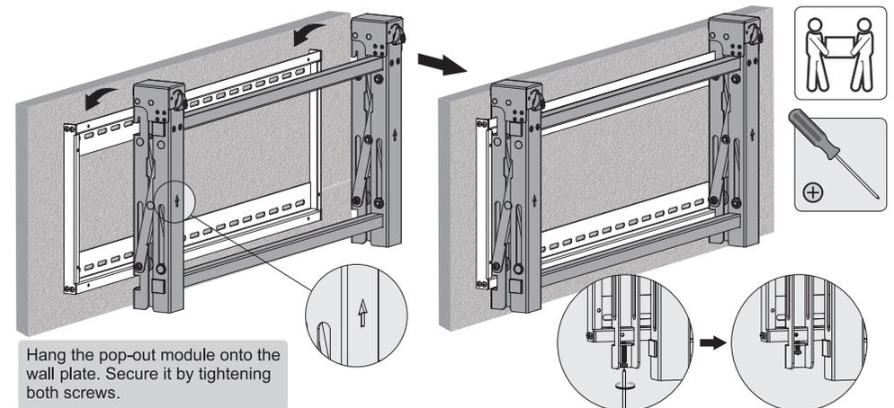
Hang the pop-out module onto the wall plate. Secure it by tightening both screws.
