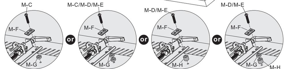
**Note:** Choose the appropriate screws, washers and spacers (if necessary) according to the type of screen.
