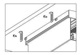
3. Place the L tighteners onto the fixing points.
