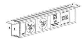
2. Attach the bracket using the provided screws according to the designated positions on the brackets
