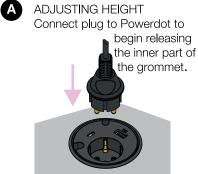
RELEASE INNER PART Rotate plug counter-clockwise to release the innert part.
