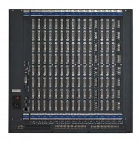
VS-6464DN-EM is a high-performance 8x8 to 64x64 modular matrix switcher chassis for AV signals. The unit is a multi-format digital switcher, populated from 8x8 to 64x64 in increments of eight inputs and/or eight outputs. The chassis includes two power supplies with an optional third for redundancy, a control module and a test module that can monitor and test any input and output in the matrix. VS-6464DN-EM supports a wide variety of input and output cards for different AV signals
