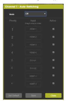
Figure 31: Routing & Scaling Page - Auto Switching Window
