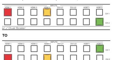
When in the Transition mode, pressing the ENTER front panel button in the Follow mode will switch the CH 1 inputs to follow the CH 2 inputs:
