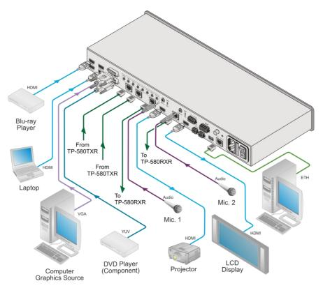
Figure 3: Connecting the VP-778 Presentation Matrix Switcher/Dual Scaler
