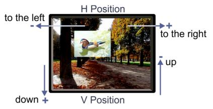
Figure 16: Positioning the Window
