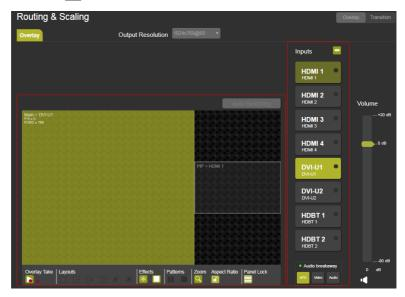
Figure 42: Routing and Scaling Page - Overlay Take
