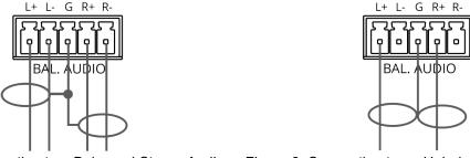
Figure 5: Connecting to a Balanced Stereo Audio Acceptor
