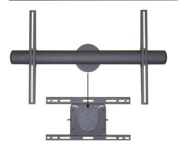
6. Lower the universal bracket bar with attached display into the cradle (as shown to the left).
