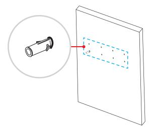
3. Position the wall mount on the wall. Then secure the wall mount with eight screws (**B**) through the washers into the installed anchors on the wall.
