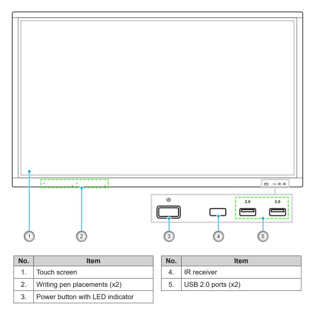
**Note:** The front USB 2.0 ports are full channel USB ports. USB ports can be used irrespective of the chosen input source.
