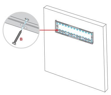
4. Align and hook the dual mounting brackets to the wall mount.
