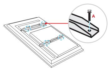
2. Drill eight small holes on the mounting location and insert the anchors into the holes.
