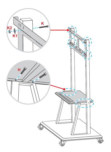
7. Align and hook the dual mounting brackets to the installed wall mount on the stand poles.
