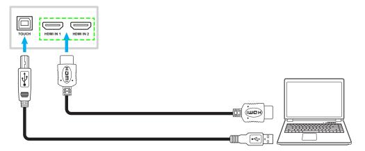
• Connect your video source to the device using an HDMI cable.
