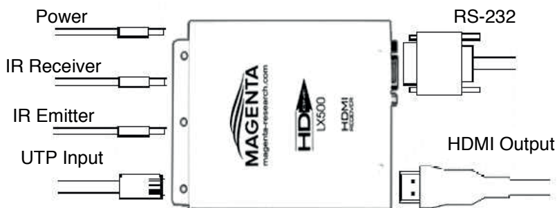
Figure 3-2. Connections on the Receiver
