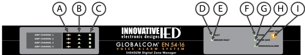
Figure 3-2: 5404DZM Front Panel Indicators and Controls
