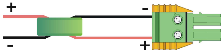
Fig. 6. Mounting the ferrite cores on the DC cables to the amplifiers
