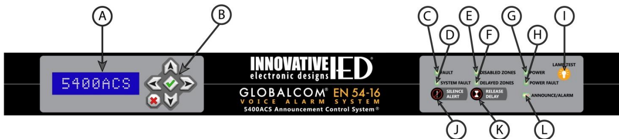
Figure 2-2: 5400ACS Front Controls and Indicators
