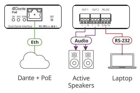
Figure 3: Connecting to the FC-101Net Rear Panel
