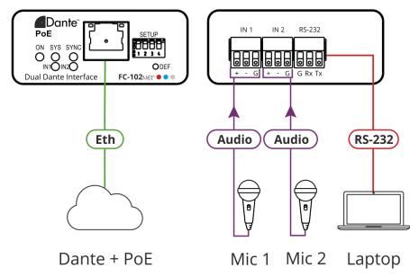
Figure 4: Connecting to the FC-102Net Rear Panel
