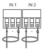
Figure 6: Connecting an Unbalanced Stereo Audio Source to the Input
