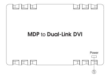
① Power LED: When the USB cable is connected with power supply this power LED will illuminate in red.
