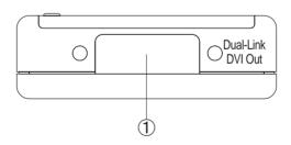
① Dual-Link DVI Out: Connect This slot is to connect with DVI display for output image with Dual-Link DVI cable.
