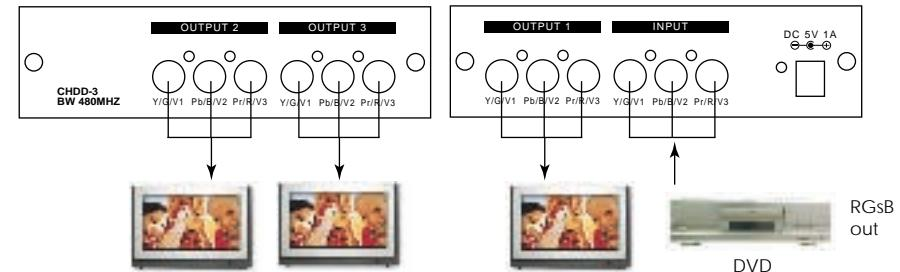
3. Works as a three 1-in 3-out distribution amplifier for composite video source.
