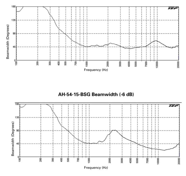
AH-54-15-BSG Horizontal Beamwidth (-6 dB)
