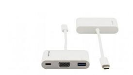
Kramer's ADC-U31C/M1 is a USB 3.1 Type-C to multiport adapter cable, supporting 1920 x 1200 or 1080p at 60Hz on the VGA video output to any VGA display or projector.
