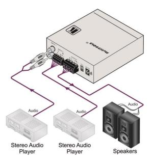
Figure 2: Connecting the 907xl Power Amplifier/Mixer
