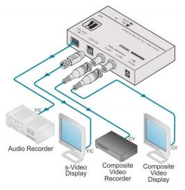
Figure 2: Connecting the 810 Color Bar/Audio Generator
