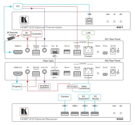
Figure 3: Connecting the 691 and 692
