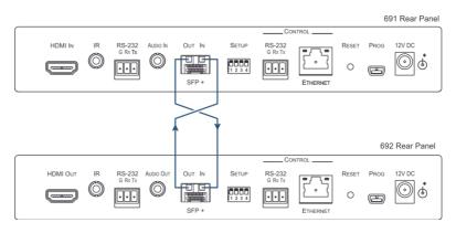
Figure 4: Connecting the Fiber Optic Cable
