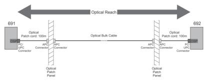
Figure 5: System Layout Example for Optical Reach Evaluation
