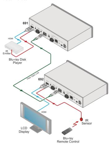
Figure 12: Controlling a Blu-ray Disk Player via the 692 Receiver
