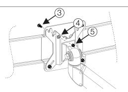
Place the LCD monitor face down on a flat surface. Align the VESA
