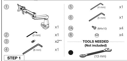
1 Use the 2 mm Allen key 2 to loosen the screw that is keeping the arms of the monitor arm 1 in the clamp and remove it as seen in the illustration. Put the arm and hexagon cup point screw 3 aside somewhere close as it will be re-inserted for STEP 3.
