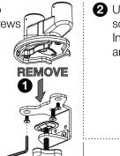
2 Use the same three screws to fasten the In-Desk bracket 3 and long bolt B2.
