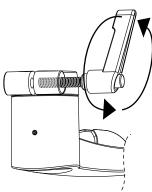
1 Unscrew and position the handle bolt so that the bolt only has contact with one half of the plastic clamp.
