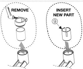
4 Remove the black plastic clamp and replace the old bushing with the one provided in the carton box 9. Repeat process with the second arm(8).
