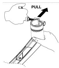
3 As the bottom part of the black plastic surfaces; pull lever outwards until the clamp is completely loose.
