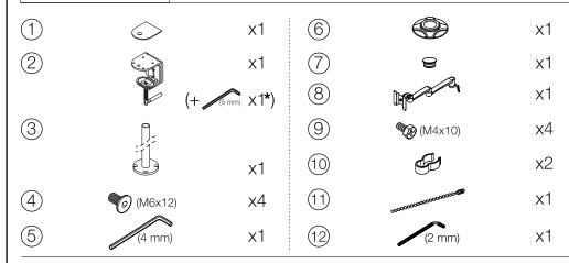
1 Adhere pad(1) to the bottom side of the clamp(2). Fasten clamp to the table using the handle. Mount the pole on top, using the screws 4 Once the pole is and Allen key(5). Complete assembly fastened, attach with plastic covers (6) & (7) both plastic covers (6) & (7) 1 Adhere to the pole. pad
