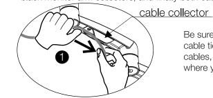
Be sure to use the cable tie (1) to collect cables. where you deem fit.
