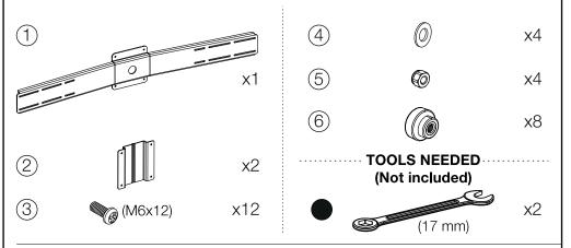
2 Mount the Dual bar 1 to the monitor arm 6. Lift the bar into position by aligning the VESA holes and pass the screws 3 through one by one. If necessary use the washers 4 and fasten using the nuts 5.
