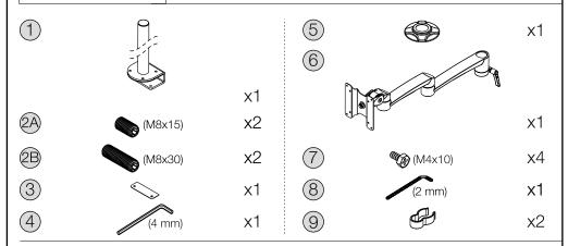
Position and mount the clamp① to the table. For tables thinner than 21 mm, use screws②B. Position the metal sheet③ and fasten it using the screws and Allen key④ (See illustration).
