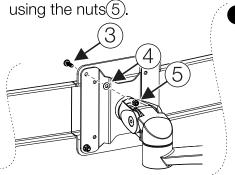
Be sure to tighten the nut of the monitor arm using an extending wheel nut wrench in order to prevent rotation of the dual bar.
