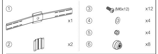
1 Mount the Dual bar(1) to an appropriate monitor arm. Lift the bar into position by aligning the VESA holes and pass the screws (3) through one by one. If necessary use the washers (4) and fasten
