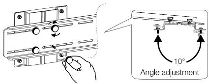
4 The Dual bar should now be fully assembled. Make sure the monitor screens are as close to each other as possible by making small adjustments.
