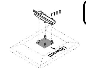
•These screws (M4/15L) are just for special monitor when the original screws are too short to fasten.
