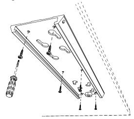
4 Be sure to insert the sleigh module, (e.g Laptop holder), into the track, before putting the spring pin② and the LIFTSYSTEM™ cover④ back to their respective positions.
