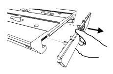
2 Examine the illustration below and proceed with the removal of the spring pin2. Remove from holes in two steps:
